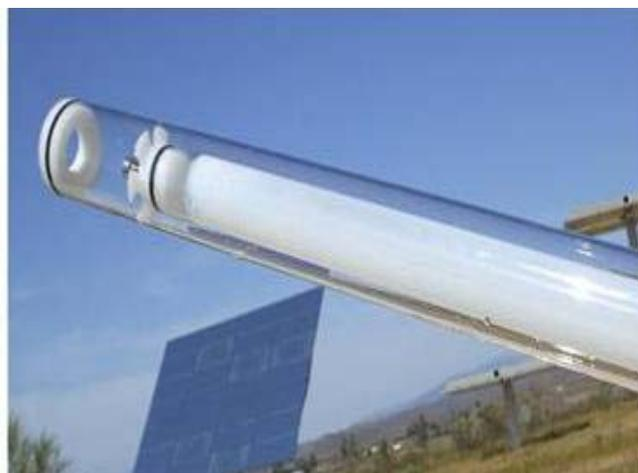
**Figure 1:** Immobilised nano-titania particle used within the SODISWATER project pilot scale solar-photocatalytic disinfection apparatus, which was developed during the EU funded project.
