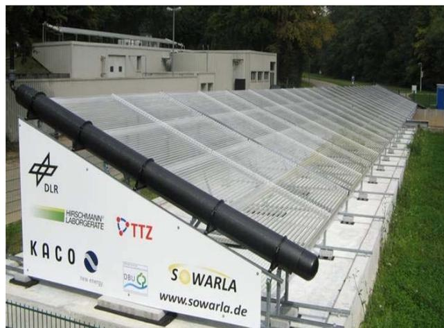
**Figure 2:** RayWOx solar receiver by Hirschmann for solar photocatalytic water purification.
