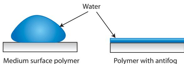
Anti-fog flattens the droplets of layer in a thin, transparent layer
